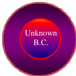
The Cauchy problem for the identification of BC inside a pipe with overspecified B.C at the external boundary. Transient heat conduction
